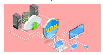
A remote access solution allows the possibility of establishing what is called a VPN (Virtual Private Network) between remote devices and the organization's network. It creates a secure extension (by establishing an IPSec or SSL tunnel) of the organization's local area network (LAN) over a public and, by default, insecure network such as the internet. There are
